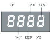
N.C. inputs are represented by the vertical segments. N.O. inputs are represented by the horizontal segments.
